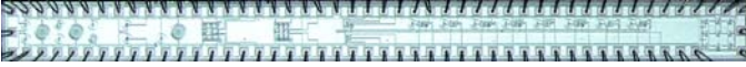
Figure 2. First array chip, designated AE-189. The chip contains three nine-element arrays, and eight active quenching circuits. The arrays have 60, 80 and 150-micron spacing; each array has two independent elements and seven summed elements. Test pixels with various sizes are included on the left.
