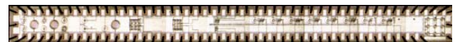
Figure 2: Photograph of CMOS APD chip that contains three nine-element arrays, and eight active quenching circuits. The arrays have 60-, 80- and 150- \mu\text{m} spacing; each array has two independent elements and seven summed elements. Test pixels with various sizes are included on the left.
