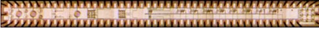
Figure 2. First array chip, designated AE-189. The chip contains three nine-element arrays, and eight active quenching circuits. The arrays have 60, 80 and 150-micron spacing; each array has two independent elements and seven summed elements. Test pixels with various sizes are included on the left.
